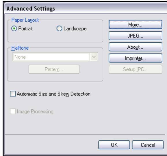
3. From here, the path to access the endorser features depends on the scanner driver. In this example a Fujitsu fi-5650 is being used. To access the endorser feature of the Fujitsu fi-5650, click on the “Imprinter” button and check the Enable box in the upper left hand corner.
