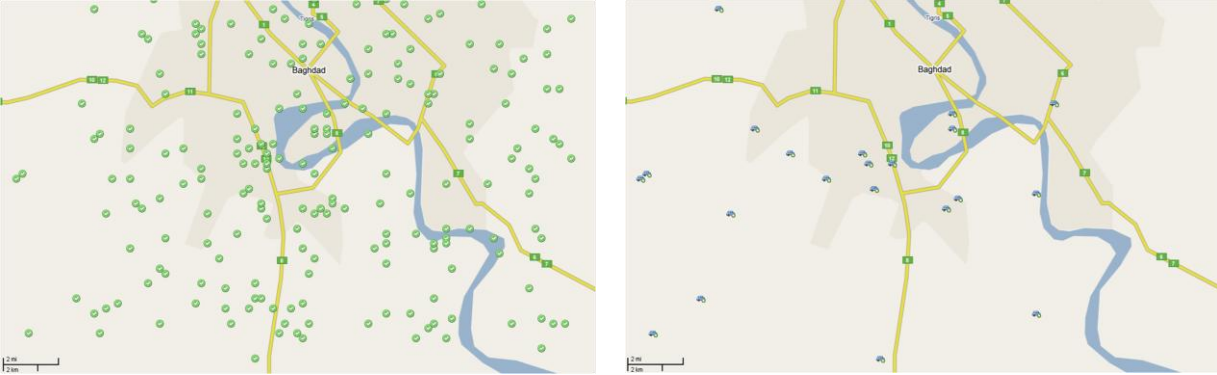
Fig. 4. These screenshots show the original 200 events (left) and the results after filtering the semantically enriched events for vehicle thefts (right). The resulting events are projected as icons onto a map of the AOR for analysts to examine. Selecting an event icon causes the message details and the semantic metadata to be displayed.
