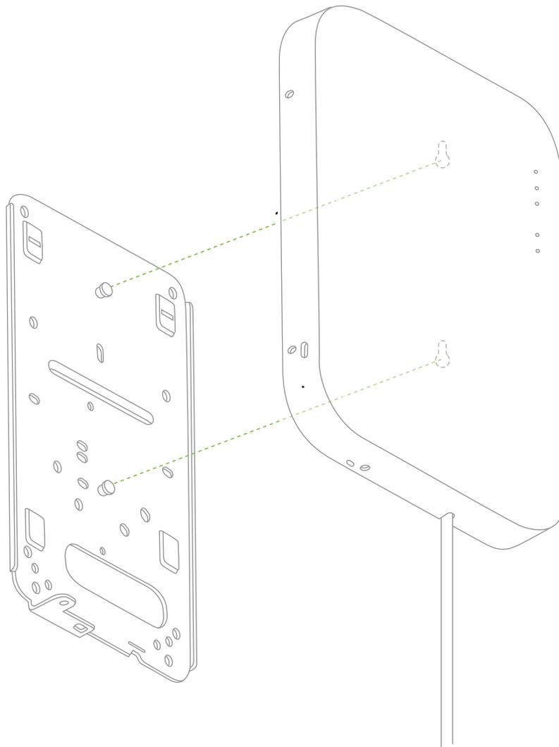
To line the access point mounting posts up with the mount plate attachment slots properly, line up the bottom edge of the AP with the horizontal slit in the mount plate. Then line up the black screw on the bottom surface of the AP with the triangular cutout in the mount plate. The mounting posts should now align with the attachment slots. Slide the unit down until it clicks into place.
