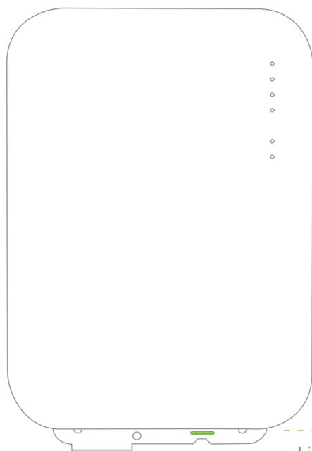
Line up bottom edge of AP with slit in mount plate
