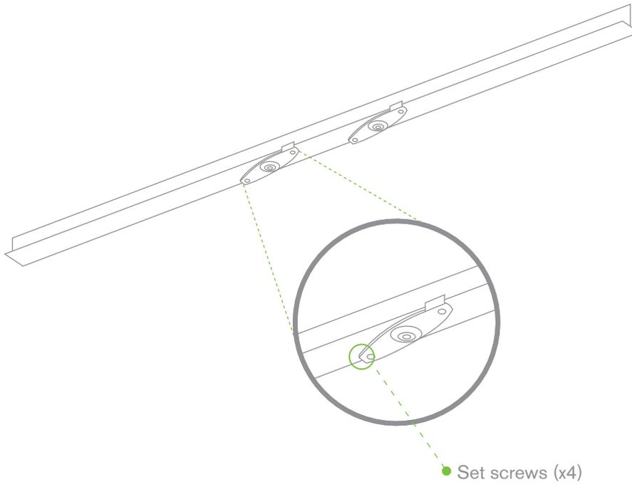
4. Attach the mount plate to the T-rail clips using the mount plate holes (marked with a "T").
