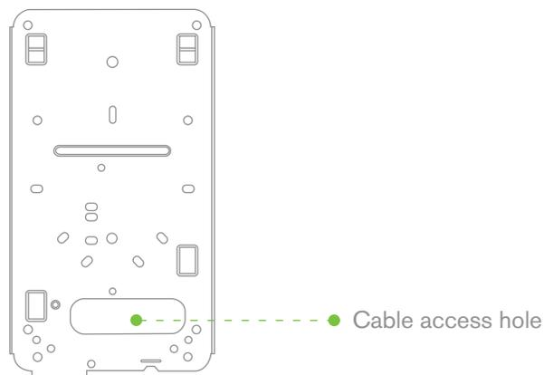
If mounting to a wall or ceiling, the Ethernet cable will feed through the cable slot on bottom of the MR24.
