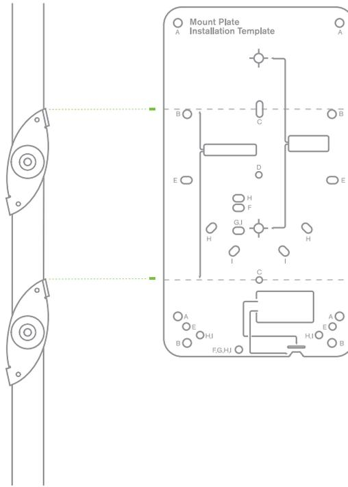
3. Tighten the set screws on the T-rail clips to secure the clips using a 5/64"(2 mm) hex key.
