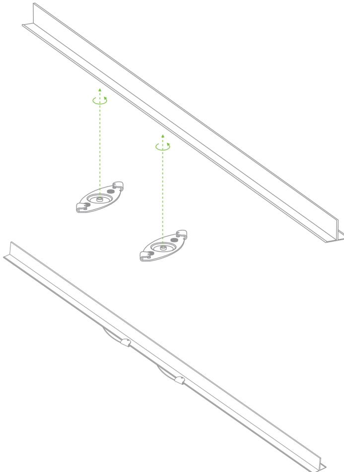
2. Using the dashed lines on the mount plate template as a guide, set the proper spacing of the T-rail clips on the T-rail
