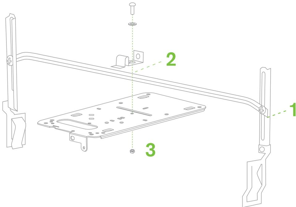
4. Securely attach the clips on either side of the T-bar box hanger to the suspended ceiling grid T-rails.
