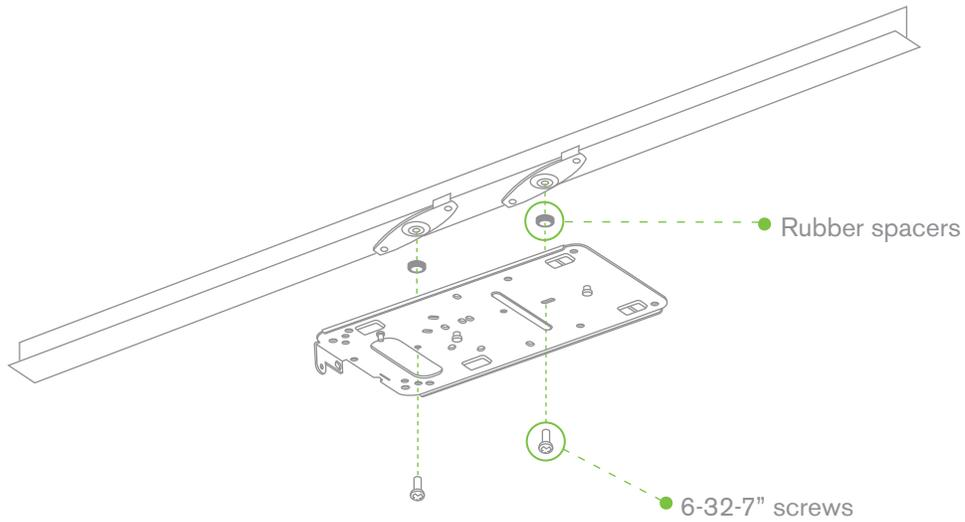
**!** **Tip:** Pre-assemble rubber spacers and screws to the mount plate. The mount plate can then be held with one hand while the other hand holds a screwdriver.
