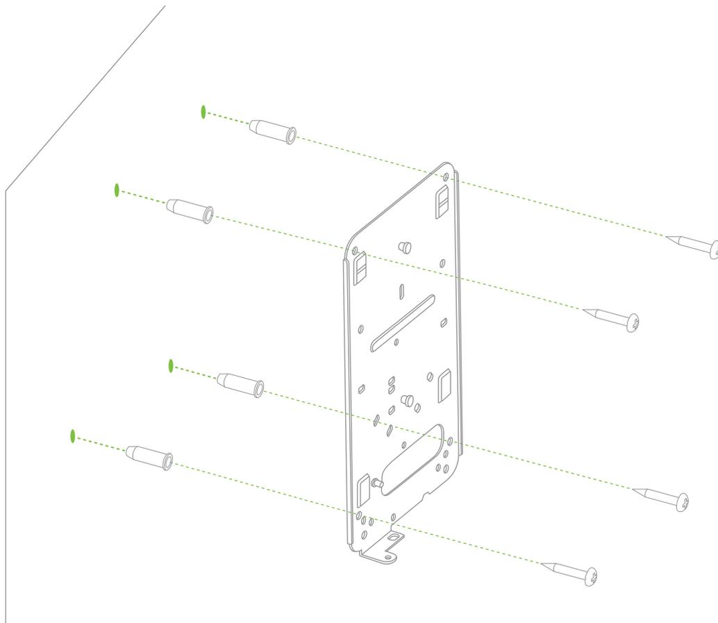
It is recommended that the MR24 be mounted to a wall or solid ceiling using the mount plate for physical security reasons.
