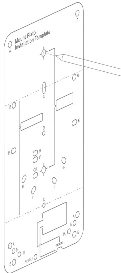
Install appropriate screws in the wall at the marked locations. Maximum screw head diameter should be 0.22" (5.5 mm). Leave approximately 0.3" (7.5 mm) of screw sticking out of the wall.
