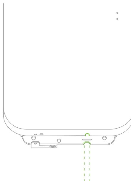
Line up cable notch in AP with notch in mount plate
