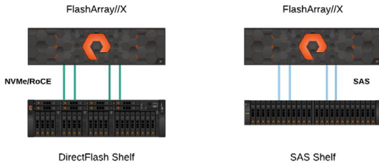
FIGURE 1. FlashArray with DirectFlash and disk shelves
