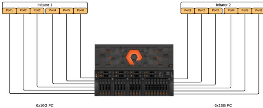
FIGURE 3. Baseline test setup – Fibre Channel
