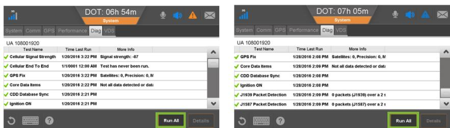
2. Confirm ✓ for Cellular Signal Strength, Cellular End to End, GPS, Core Data Items, Ignition ON, and CDD Database Synch. J1939 and J1587 are dependent on databus connections, at least one of these tests must pass. If they do not, talk to your dispatcher.
